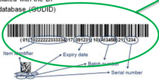
Fig 3: Alternative example of UDI illustrating DI and PI requirements in order to comply with new FDA UDI regulations
