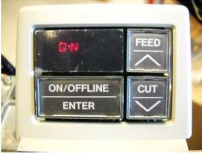
This printer has 2 modes: ONLINE (ON will be displayed on the screen) and OFFLINE (OFF will be displayed on the screen). The printer must be in the ONLINE mode in order to receive print commands, and also to print. The printer must be in OFFLINE mode in order to access the special functions, commands, and to access the menu system. The menu system will be explained in much greater detail in the following section.
